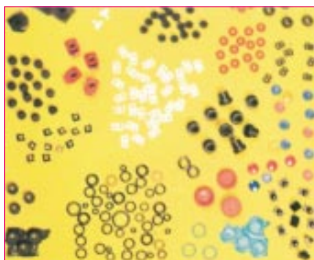
Parts before and after deflashing by a oscillating deflashing machine (model MPCD)
